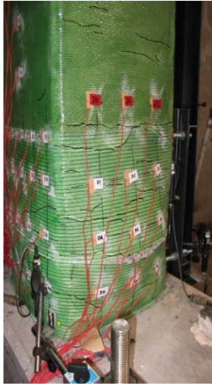
Figure 6: High plastic deformation with PET fiber
