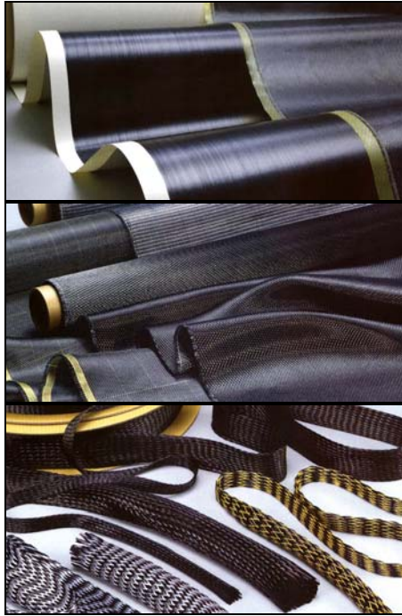
Figure 5: Unidirectional carbon fiber ply and random mat (top); woven carbon fabrics (middle); and braided hybrid fibers (bottom) [29].
