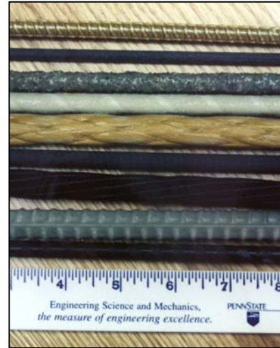
Figure 10: Examples of FRP bars and tendons. Scale is in inches (1 inch = 2.54 cm).
