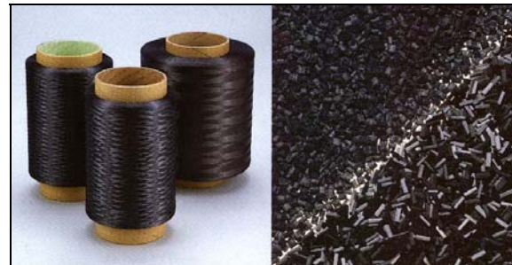
Figure 4: Spooled continuous carbon fiber (left) and short chopped carbon fiber (right) [29].
