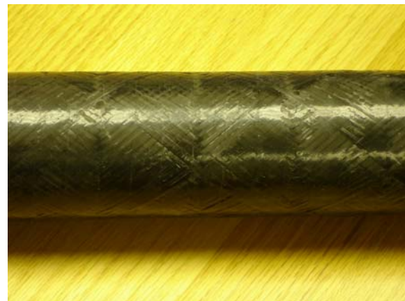
Figure 14: Small-scale example of a helically wound carbon FRP tube with fibers at \pm 40 -degrees relative to the longitudinal axis.
