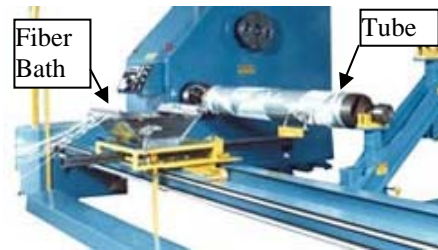
Figure 13: Example of FPR tube winding with a filament winder [37].
