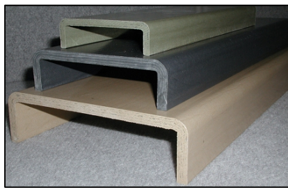
Figure 9: Examples of FRP structural shapes made by pultrusion [35].
